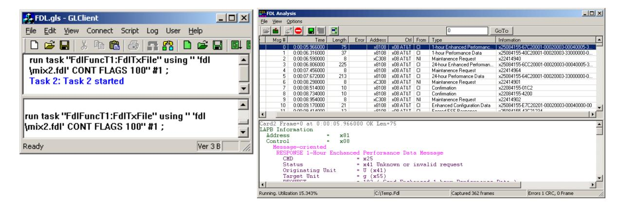
Receive and transmit HDLC frames and signals in \*.hdl file format over facility data link (FDL)
