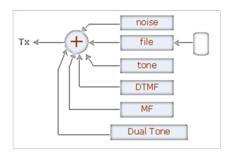
Digitally synthesized generators of tone, noise, DTMF digits, MF digits, and dual tone are summed and transmitted into timeslot
