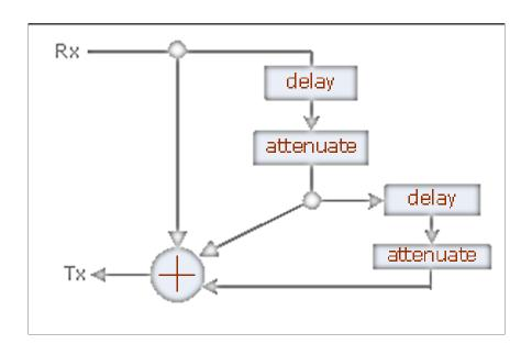
Three parallel echo paths are summed with a digitally synthesized tone and noise and a PCM file, a more complex structure for echo path modelling
