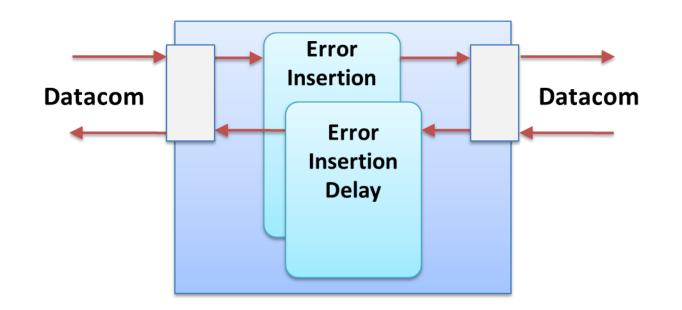
• Permits inserting single, fixed, automatic, random, and burst error into the incoming bit stream
