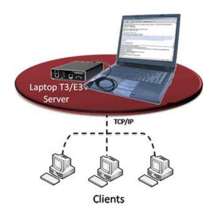
• GL's Windows Client/Server software is a non-GUI based program for remote, scripted, and automated control of T3/E3 configuration, capture, transmission and more.
