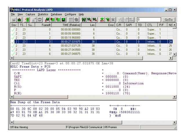
GL's T3 (DS3)/E3 analyzer supports protocol decoding and analysis of ATM, Frame Relay, PPP, and HDLC. All the protocol analyzers are based on similar architecture and supports sophisticated filtering, statistics and real-time capture options
