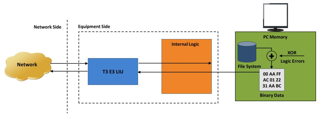
• The transmit file application permits transmission of a file of any length or transmission of data from memory in hex format
