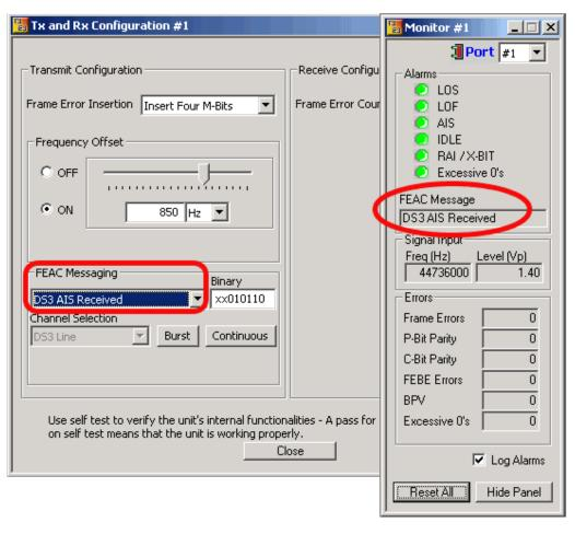
Using the FEAC channel, alarm or status information from the far-end terminal can be sent back to the near-end terminal. The Monitor T3 Line indicates the incoming FEAC message
