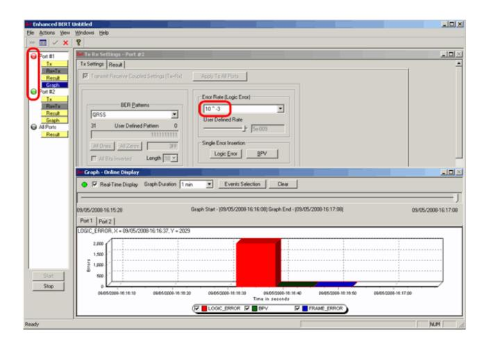
GL's T3 E3 Bit Error Rate Tester application measures the correctness of data received on T3 E3 channels for a repetitive fixed or pseudorandom pattern for the given transmission
