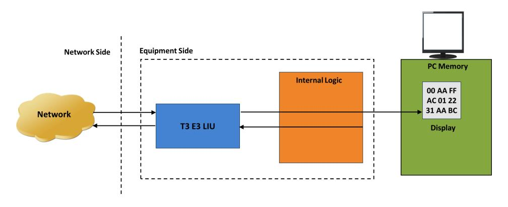
This application can monitor raw bit values on the selected ports. The raw bytes received from the network at the T3 interface are monitored and displayed on the selected ports
