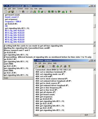
Allow the user (with an appropriate client) to operate analyzers remotely, write scripts for automation, or provide multi client connectivity to a single T1 E1 VF Data analyzer
