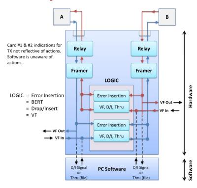
• Used for Drop and Insert applications in which the board analyzes the traffic running between two pieces of T1 E1 equipment. This feature also eliminates complex cabling
