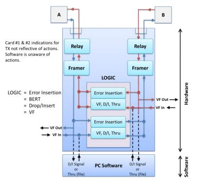
Used for Drop and Insert applications in which the board analyzes the traffic running between two pieces of T1 E1 equipment. This feature also eliminates complex cabling
