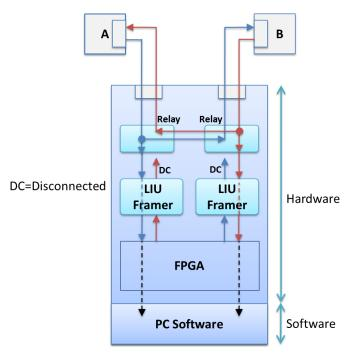
• This mode is similar to the standard "Outward Loopback" which allows monitoring T1 E1 lines "in-line" while still being protected from loss of power to the board
