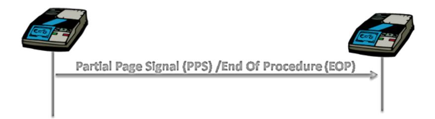
After the T.4 transmission and the subsequent return to control mode, the sending device must send one of the following signals:
