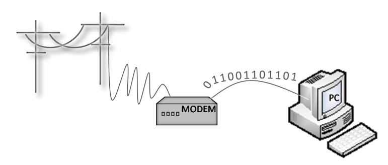
Short for modulator-demodulator. A modem is a device or program that enables a computer to transmit data over, for example, telephone or cable lines. Computer information is stored digitally, whereas information transmitted over telephone lines is transmitted in the form of analog waves. A modem converts between these two forms.
