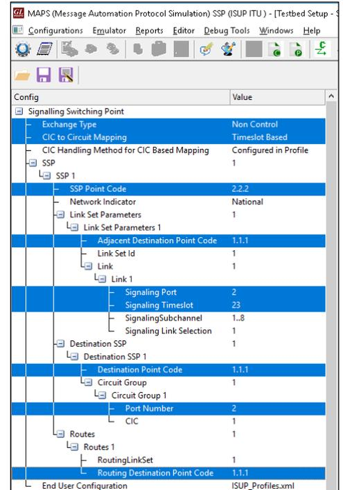
**Note:** In **Testbed**, User can enter **OPC** and **DPC** Point Codes in the **Dotted Decimal** or equivalent **Decimal/Hexadecimal** format.
