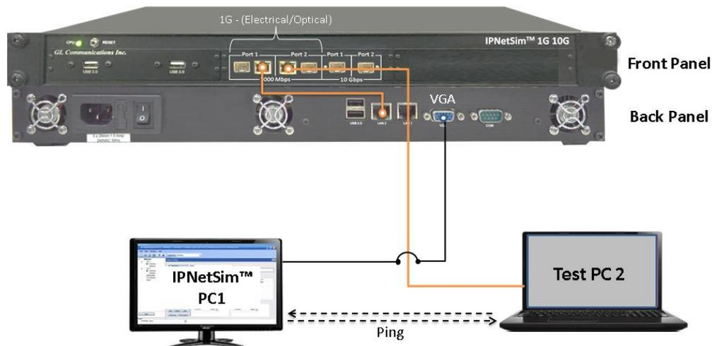
The IPNetSim™ application and the related license are pre-installed on the rack PC. Plug the monitor and get started with the application as explained in the steps below.
