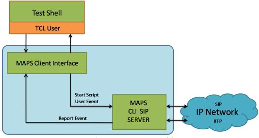
Figure: SIP Test System Modules
