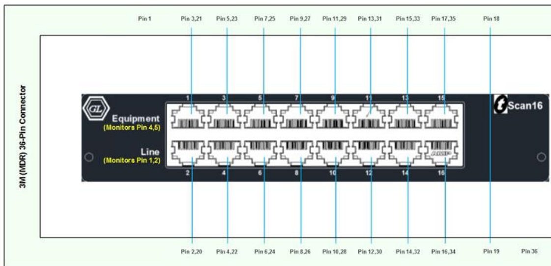
Figure 4: Pin-to-Pin Connection between the Breakout Box and the tScan16™
