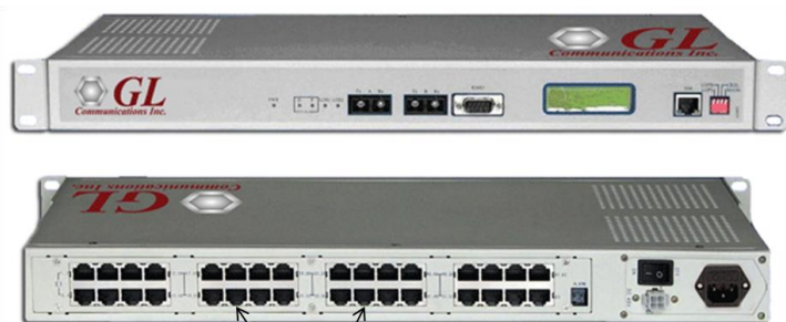
Each RJ-45 provides 2 full duplex E1 interfaces
