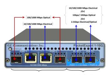
Port#1 and Port#2 10/100/1000Mbps Electrical (Or) 100/1000Mbps Optical Ports Port#3 and Port#4 10/100/1000Mbps Electrical (*Or*) 1G Optical Ports (*Or*)
