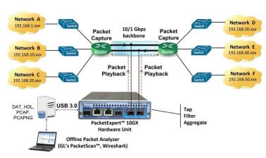
**Wirespeed Ethernet Packet Capture and Playback**
