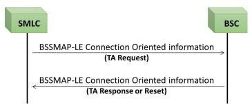
**Figure: TA Positioning Procedure**
