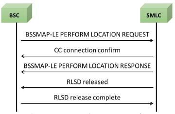
**Figure: BSSAP-LE Location Request Procedure**
