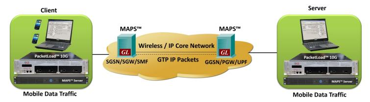
GL's MAPS™ Server with PacketLoad™ appliance supports massive simulation of UEs (up to 100000) with mobile data traffic at very high speed rates (up to 4 Gbps or 40 Gbps) over LTE IMS network.
