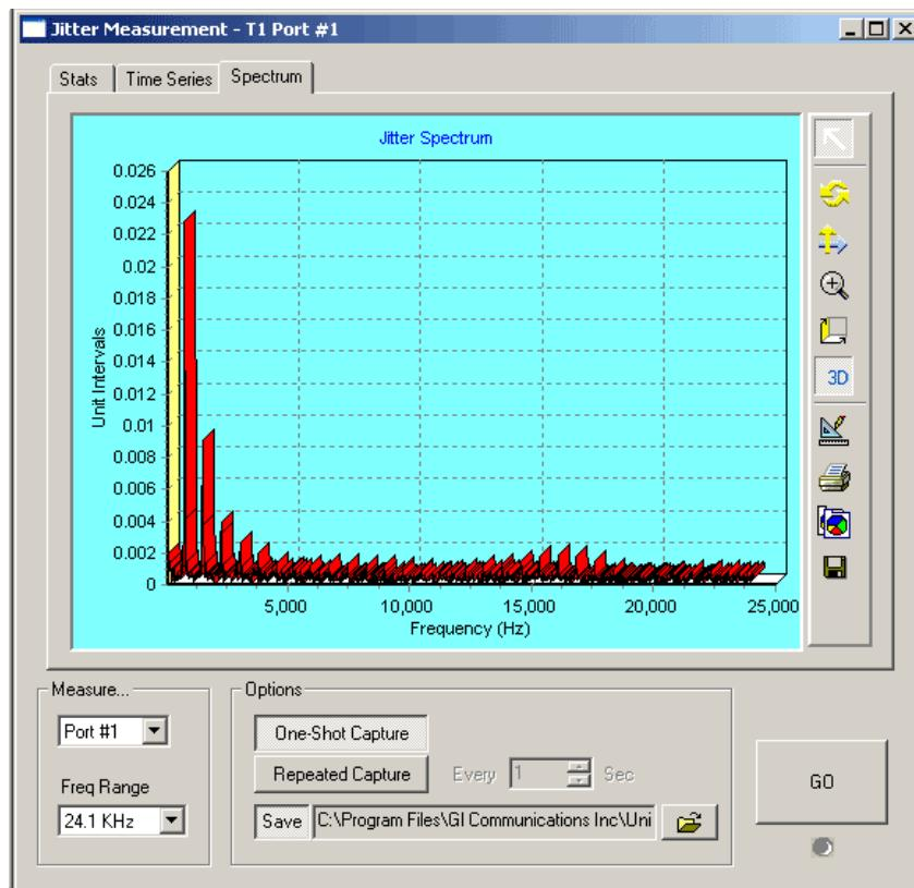
Jitter Measurement for T1 E1 Signals
