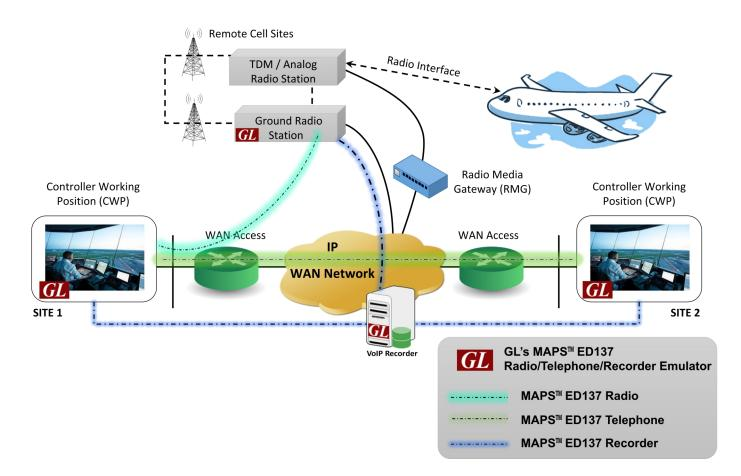
Voice communications for Air Traffic Management (ATM), whether it is **Air-Ground (AG)** or **Ground-Ground (GG)** were predominantly over TDM based ATM networks. With the latest developments in EUROCAE (European Organization for Civil Aviation Equipment) ED137 inter-operability standard, it is now possible to implement VoIP technology for air traffic control communications.
