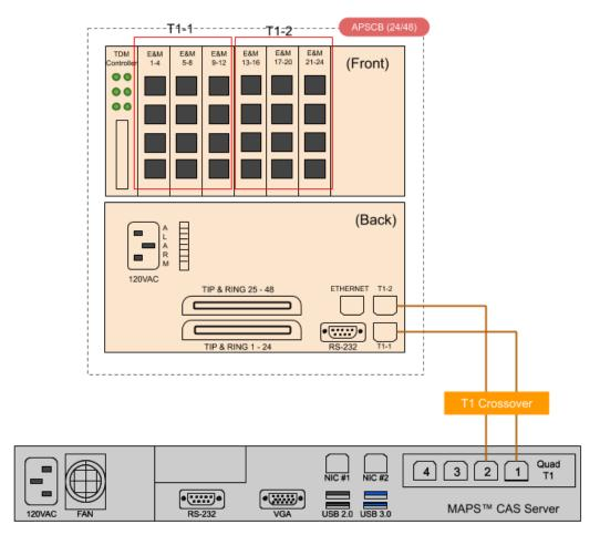
Each E&M service card provides four female RJ-45 connectors. Each T1 supports 3 E&M service cards for a total of 12 E&M interfaces.
